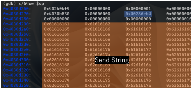
Fig. 12. Stack area of ARM64 environment after executing the exploit code (the area in the orange frame is the buffer, and the area in the blue frame is the return address)
